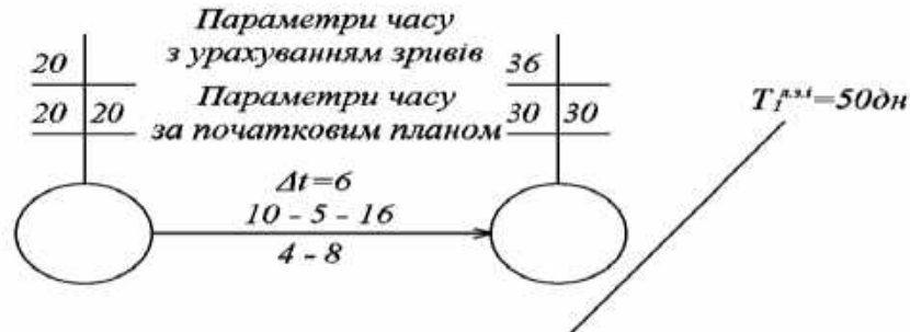
Fig. 1. An example of recording time parameters of a network graph taking into account disruptions to the line of information capture.
