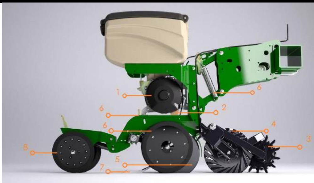
Fig. 1. Section of the seeder of precision seeding: 1 – construction of the seeding device, 2 – vas deferens, 3 – unfolders, 4 – turbodisc, 5 – opener, 6 – sowing depth adjustment system, 7 – seed sealer, 8 – rolling wheels
