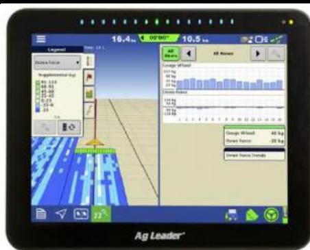
Fig. 8. InCommand 1200 AgLeader monitor.
